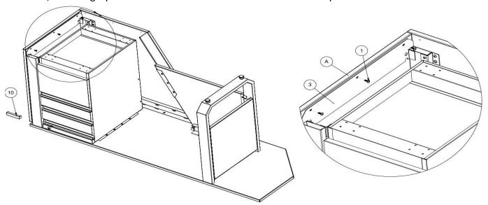
17. Place item #14 between the bottom of 19179/19178 and the casters that came with 19179/19178. Install the 16x fasteners that came with 19179/19178.
