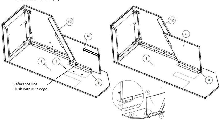
12. Place the previously assembled item #1 and panel B as shown. Attach item #8 using 2x fastener #1 to panel G and attached item #8 to item #1 using 2x fastener #3, finger tighten only. Confirm the gap between item #1 and panel G is constant and as minimal as possible as shown below.
