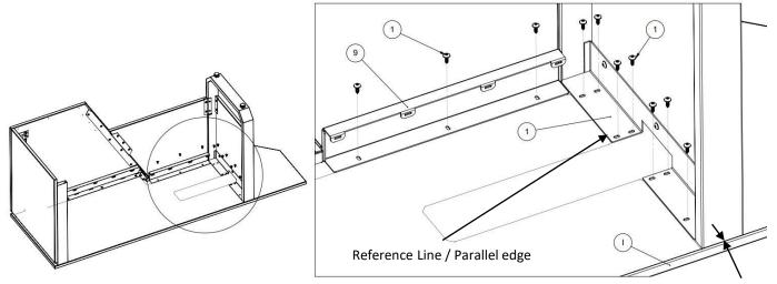
Align edge of tube from item #1 with the edge of the wood(brown surface), NOT the face of the edge banding.
