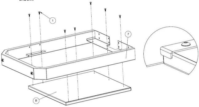
3. Place wood top on clean smooth surface upside down with the pilot holes and reference lines facing up. The reference lines will be used to help align the metal components in future steps, these are only guides final locations will vary by assembly accuracy. (Panel I is used in these instruction, substitute panel I with panel E for 60" models)
