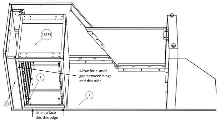
15. Place item #6 as shown, Fasten #6 to the tube of item #3 using 2x fastener #3, finger tighten only. Install 2x fastener #2. (Fastener #2 is a self drilling fastener, it will create 2 new holes in item 19179) Confirm there is a constant gap between 19179/19178 and the tube of item #3. Tighten the 2x fastener #2.
