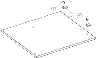
2. Position Panel B as shown, centering the panel to create equal gaps, a spacer or credit card works well. Fasten panel #7 to item A using 4x fasteners item #1 using the supplied T25 Torx bit item # 4. NOTE: The panel should sit on the metal finger as shown.
