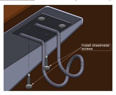
Correctly installed hook mounting plate.
