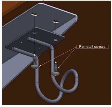
**Step 3:** Using the remaining smaller holes as a guide, install the 2 supplied self-drilling sheet metal screws using a drill equipped with a #2 phillips driver bit. The screws need to drill through the small holes, then into, and through the metal leg bracket.
