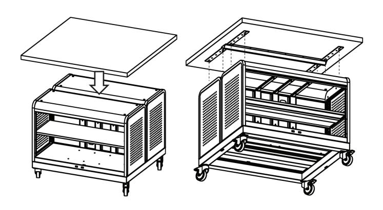
**6.** Attach the top to the cases using the  $3/8" \times 11/4"$  OD oversized washers and 3/8"-16 lock nuts with a 9/16" socket & ratchet, or 9/16" wrench.
