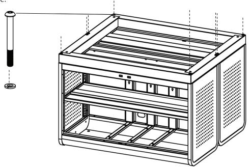
**4.** Install casters using the caster wrench provided. Hand tighten until very snug.
