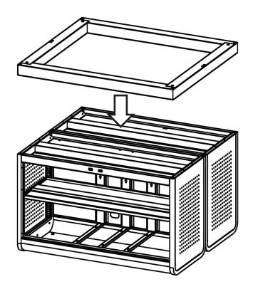
**3.** Attach the base to the cases using the 3/8"-16 x 3.5" bolts and 3/8" lock washers. **Helpful Hint:** Use clamps on the touch rails of the cases to help line up the holes with the base.
